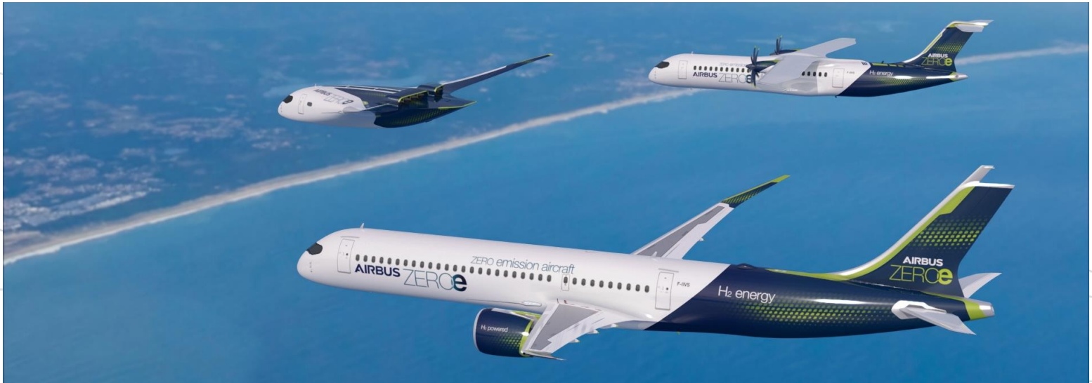
Figure 7.08 Airbus zero-emission concepts, BWB, turboprop and turbofan.
