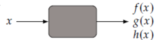
Figure 1.14 An analysis model is considered a black box when only the inputs and outputs are known.
