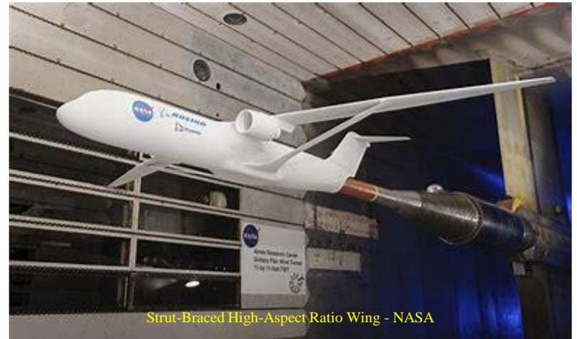
Strut-Braced High-Aspect Ratio Wing - NASA
