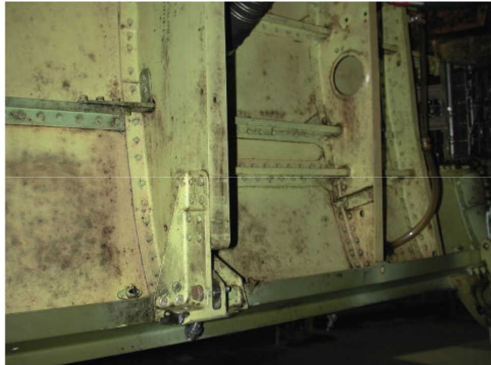
Mold originated corrosion
