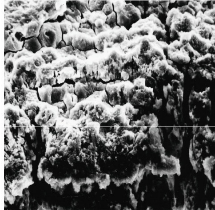
Scanning Electron Micrograph of a Corroding Aluminum Surface
