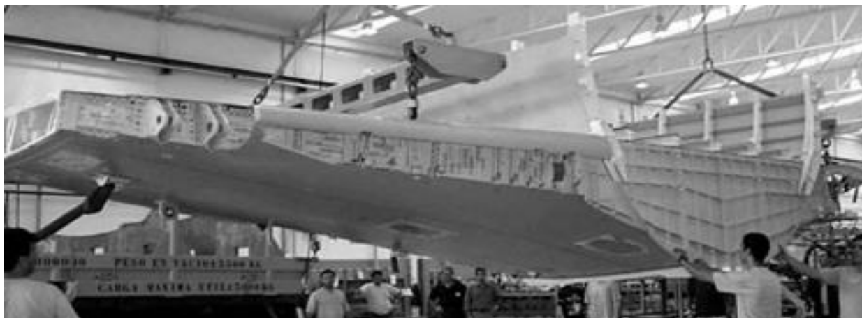
DO728 – caixão central da asa ( central wing box )
