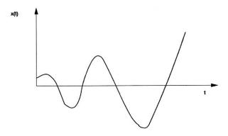
For  $c_{eff}^2 > 4k_{eff}m$  the motion is non-oscillatory and divergent:
