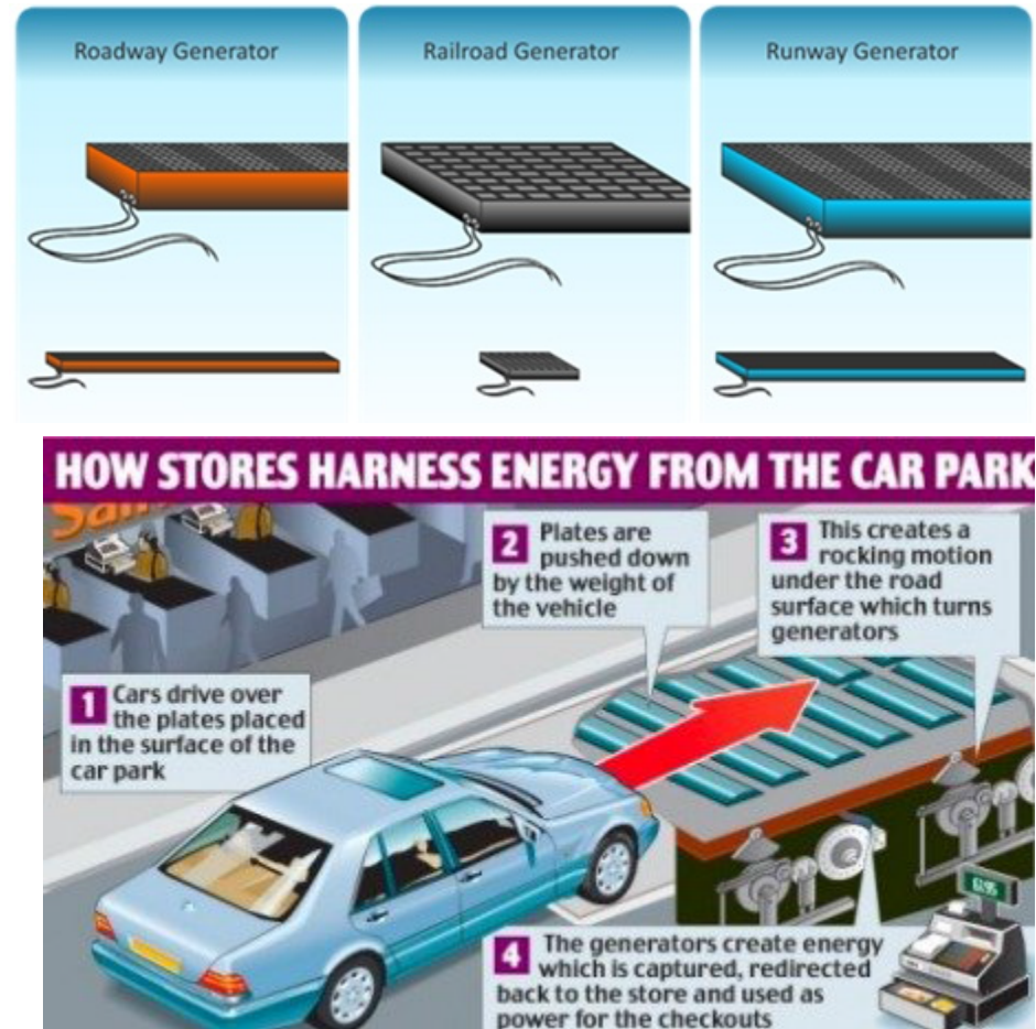
Mechanism of the power-generating floor
