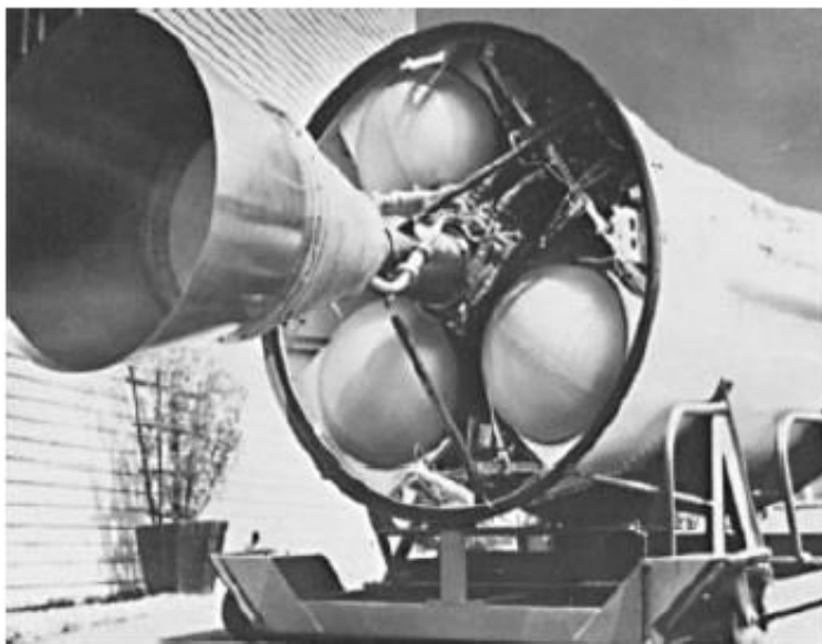
Fig. Pressure tanks manufactured from titanium for space transportation systems (TIMET, Henderson, NV, USA).
